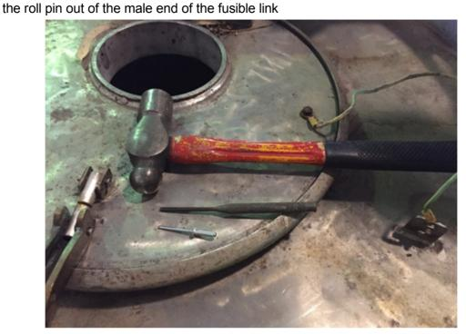
5. Hit roll pin with until flush with the bracket before using the punch or screwdriver, it will be easier to align
