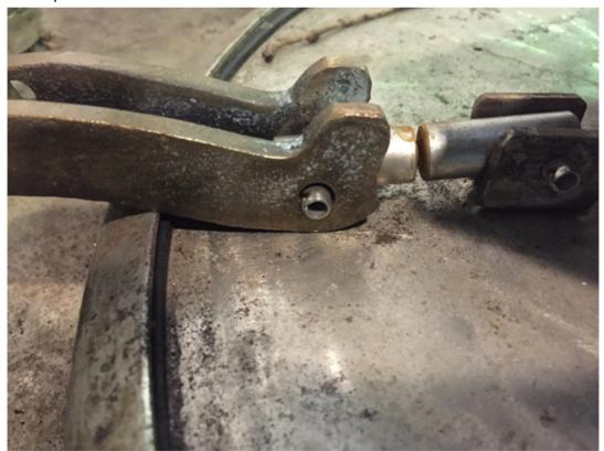
3. Determine which side of the fusible link is the male side, the thread will be fixed into this end with the solder
