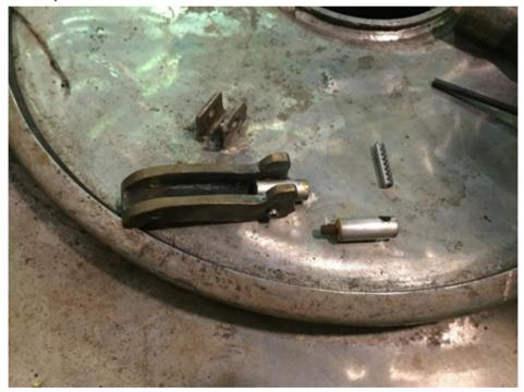
7. Drive the roll pin back into place, using a rivet or something of similar size which fits inside the roll pin will make it easier to align
